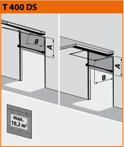
T 400 DS Elevated rail system with low spring axis A= hoisting + 200 mm B= open height – hoisting + 600 mm Width max. 3,200 mm Height max. 3,200 mm Lift min. 1,700 mm
