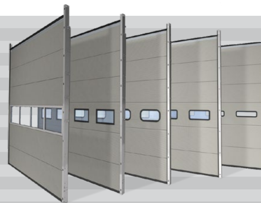
U-value ISO 40 mm sectional door: 5,000 x 5,000 mm: 1.02 W/m²K
