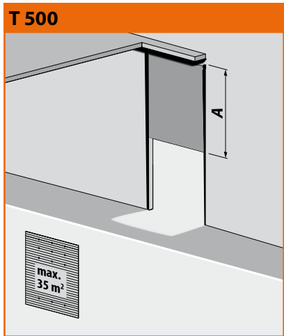
T 500 Vertical rail system A= open height + 560 mm
